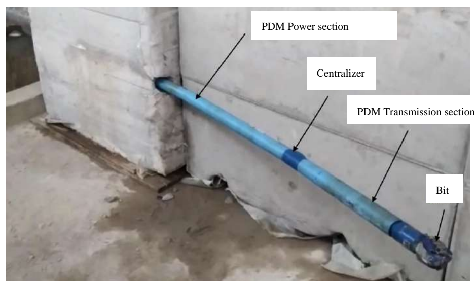
Figure 3. Photo of a two-section PDM with TS Perfobore centralizers.
