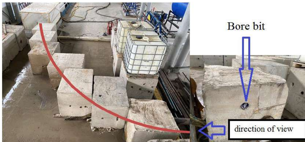
Figure 2. Bench tests of TS while drilling a channel with curvature radius of 7.7 m.
