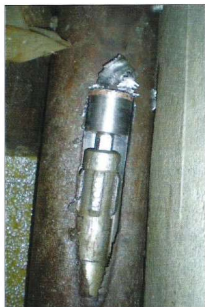
Fig. 12 Side view of the milling operation in casing
